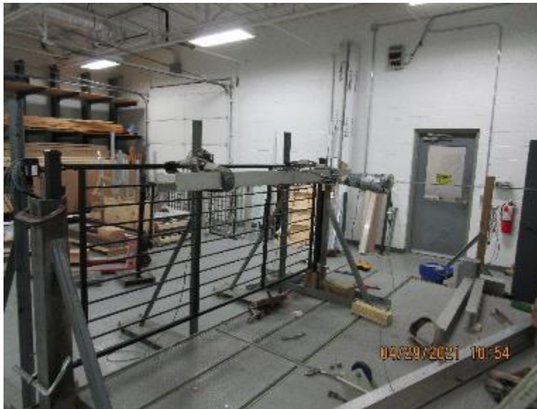
Photo No. 3 Horizontal Uniform Load on Top Rail (IBC Loading Only)
