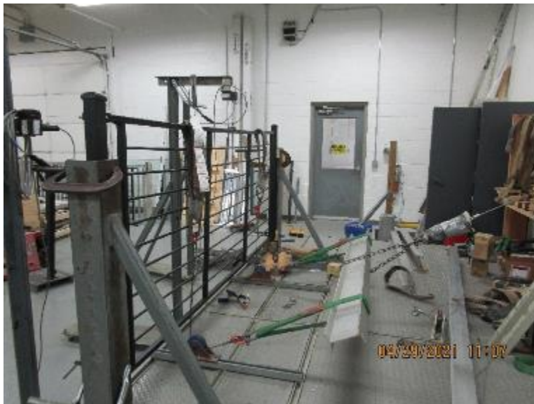
Photo No. 4 Vertical Uniform Load on Top Rail (IBC Loading Only)
