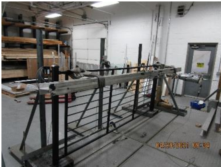
Photo No. 6 Concentrated Load Test at Ends of Top Rail (Brackets)
