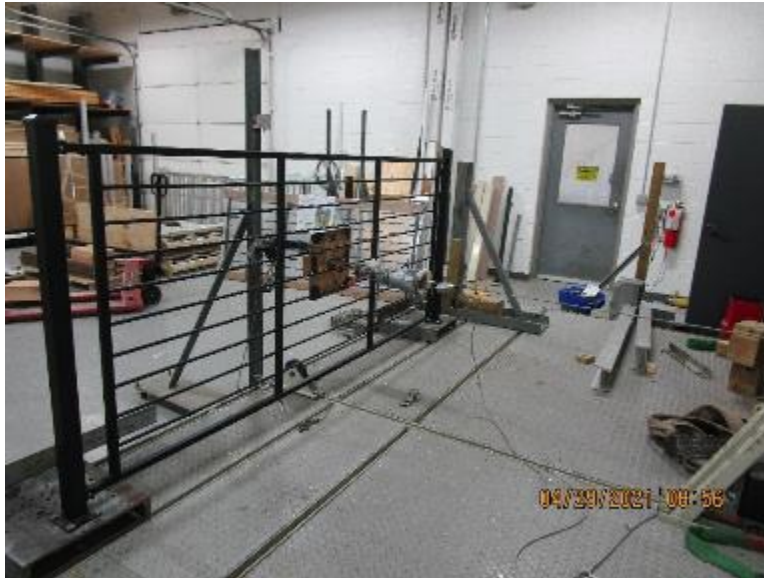
Photo No. 1 In-Fill Load Test at Center of Three Pickets
